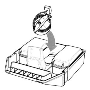
Pivot the Humminbird unit all the way down and reinstall the upper case.
