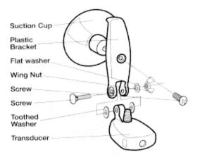
You can mount the transducer anywhere on the side of the boat if your boat remains stationary. If you are trolling, it is best to mount the transducer on the transom of the boat.
