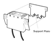
Snap the support plate to the rear of the connector holder as shown in the illustration.
