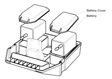
Re-install the battery covers by inserting the tab at the rear of the cover into the slot on the lower housing, and then snap the lid into place.
