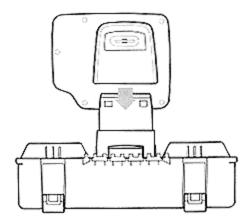
The Humminbird Portable unit is designed to use two 6-volt, lantern batteries with spring type terminals.
