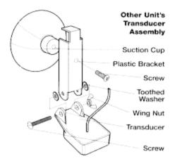
It is important that the transducer be mounted beneath the surface of the water, pointing straight down. The suction cup mount is designed for quick, easy installation and removal, not for high-speed operation. If you intend to operate your boat at any speed faster than trolling speeds, remove the suction cup transducer from the water. The transducer can cause damage or pull the portable unit into the water if it releases at high speed.
