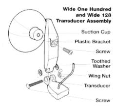
Use the bracket, which fits your transducer, and refer to one of the three following illustrations for the appropriate assembly instructions. Parts have been included for both installation procedures, so there will be some parts remaining.
