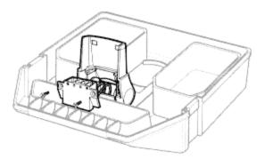
Install the Humminbird unit by sliding it onto the mounting bracket until it is fully seated. All cable connections are made automatically.
