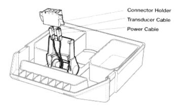
Carefully pull the excess cable from beneath the mounting surface so the connector holder aligns with the mounting holes on the front of the mounting bracket.
